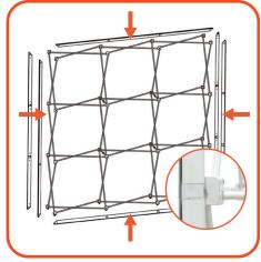
Step 5 Attach channel bars to frame. Slide channel bars onto frame from top to bottom, then secure onto metal peg.
