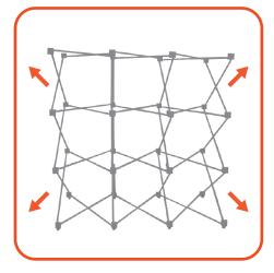
Step 1 Place frame with the adjustable feet facing down. Expand the frame.
