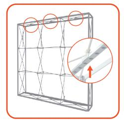
Step 7 Then snap the Edge Lights on each top middle "x" bars.
