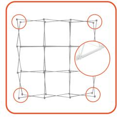
Step 3 Connect the top and bottom End Caps on each side of the frame.
