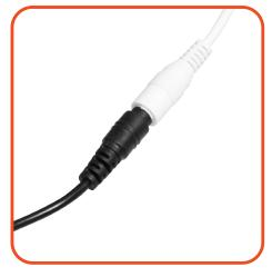
Step 9 Connect the Jumper Cord t the Transformer using the barrel connectors.
