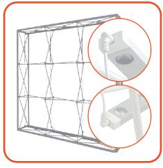
Step 8 Plus the Jumper Cords into the top and bottom Edge Lights together.
