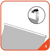
Slide the top of the graphic under the lip (it should allow for approx. 3/8" or 1cm insertion) and close the lip to secure the graphic.
