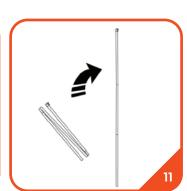
Unfold the pole and slip the pieces together to assemble it to a rigid pole (the hooked end corresponds to the top and the round end belongs to the bottom base.
