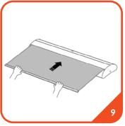
Carefully allow the graphic to recoil into the base unit (it may be useful to have an assistant hold the base steady).
