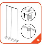
The hook at the top of the pole slips into the rear slot of the banner beam. A marker on the beam indicates the beam's center where the pole should be inserted.
