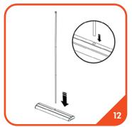
The bottom of the assembled pole slides into the round socket in the center of the base unit.
