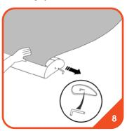
Peel off the cover, remove the screw underneath the chrome end of the base and detach. Then, with the graphic held firmly, carefully pull out the retaining pin, then put it into the cover.
