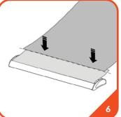
Attach Velcro strips to the bottom of the back of banner.
