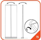
The unit can be levelled by adjusting the threaded feet at the bottom of the base unit.
