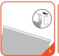
Finish the top by re-attaching the plastic end caps.
