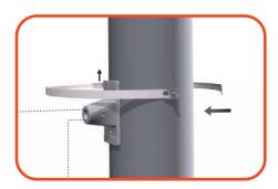
**Step 1**Place brackets on street pole and secure with stainless steel clamps
