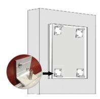
Tighten allen key screws on wall mounts to apply pressure to the frame. Repeat for all wall mounts to secure frame to the wall.
